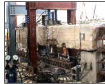
Loading test on RC beams
