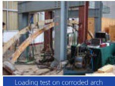
Loading test on corroded arch
